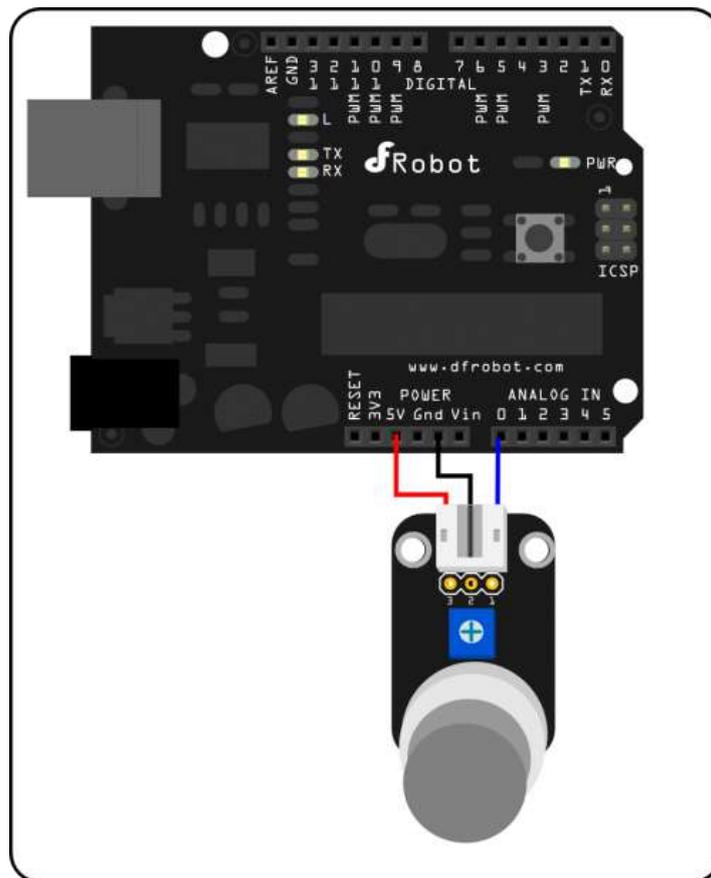
Analog sensor connection diagram
